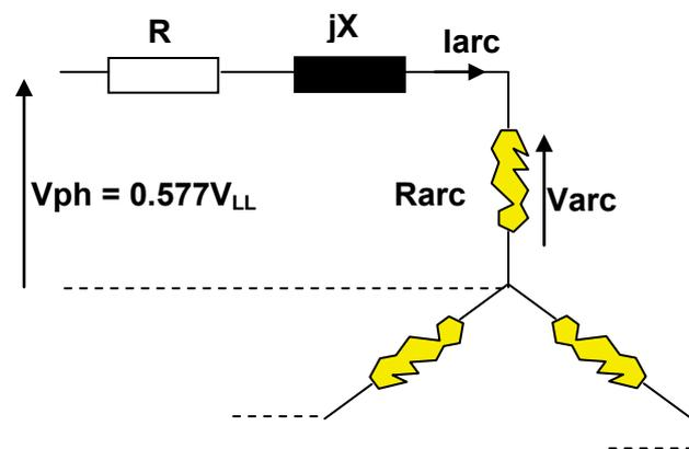
Fig. 2 Single-phase model of a 3-phase arcing fault
