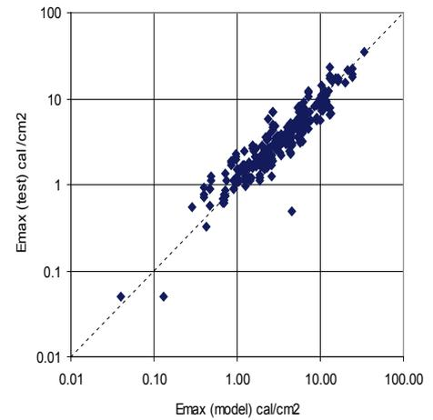
Fig.7 Comparison of calculated incident energy density with test values (all tests,  $r^2 = 0.860$ )
