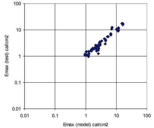
Fig.4 Comparison of calculated incident energy density with test values (open tests only)
