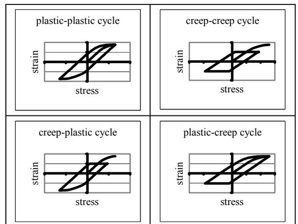
Fig. 7: Four typical cycles combining plastic strain and creep.
