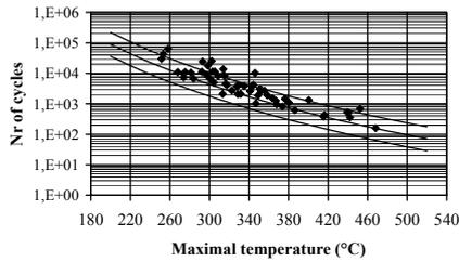
Fig.4 : Numbers of cycles are plotted versus the maximal recorded temperature, here with log-lin scale. Mean curve and 90%-tolerance-curves are also plotted.
