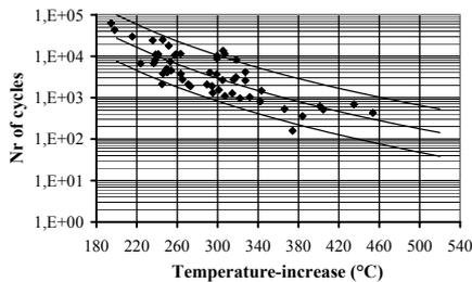
Fig.5 : Numbers of cycles are plotted versus the recorded temperature-increase, here with log-lin scale. Mean curve and 90%-tolerance-curves are also plotted.
