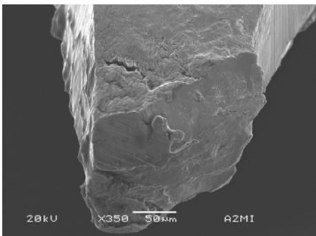
Fig. 12 : Intergranular cracking on a sample after rupture. 1200 mechanical bending-tests cycles.
