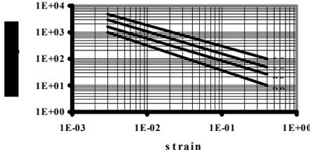
Fig. 8: For each one of the typical “plastic-creep” cycles, it is possible to estimate one ageing-law.
