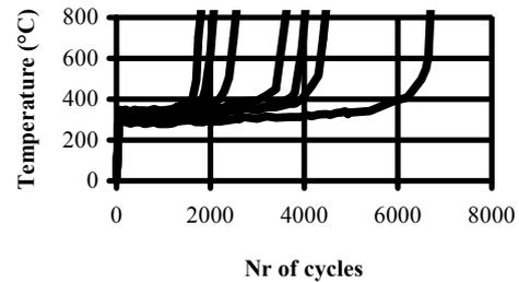
Fig.2 : Measurement of temperature through the drop voltage allows to show that the damage increases first slowly and then is accelerated at the end of life-time.
