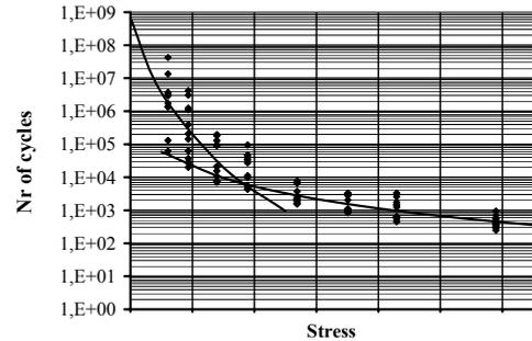
Fig.6 : Numbers of mechanical cycles are plotted versus the stress, here with log-lin scale. Two kinds of behaviour are observed according to the level of stresses.
