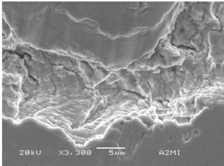
Fig. 11: Fatigue-lines on a sample after rupture. 39000 mechanical bending-tests cycles.
