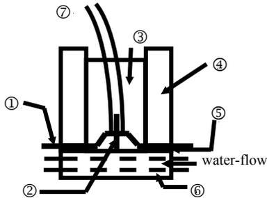
Fig.1 : Principle of the tests :①fuse-element; ②notches; ③sand; ④ceramic body; ⑤ insulating tape; ⑥water-box for cooling; ⑦drop-voltage measurement.
