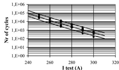
Fig.3 : Numbers of cycles are plotted versus the test-current, here with log-lin scale. Mean curve and 90%-tolerance-curves are also plotted.
