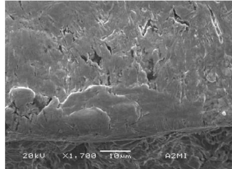
Fig. 13 : Transgranular cracking on a sample after rupture. 39000 mechanical bending-tests cycles.
