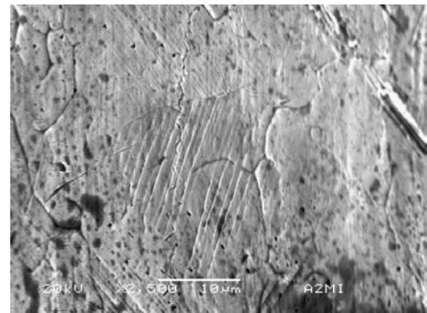
Fig. 10 : Slip-bands on a fuse-element after rupture. 450 electric cycles 1h ON/1 h OFF.
