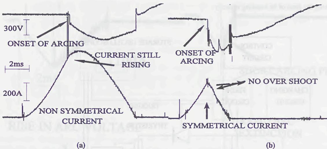
**Figure 5** Comparison of characteristics of a) 63LET Bussman fuselink and b) 63A substrate fuselink. The top trace is voltage waveform and the bottom waveform the current. The time, voltage and current scales are the same for each diagram.
