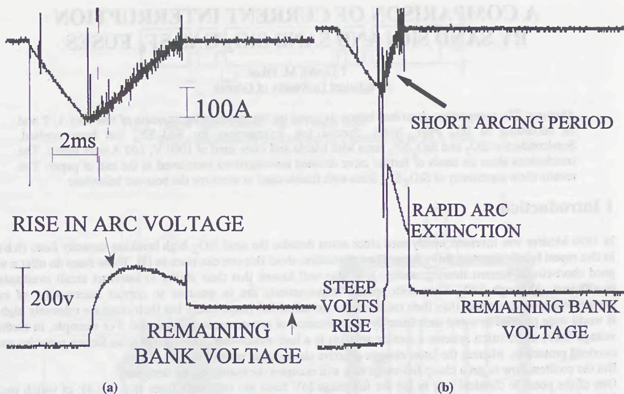
Figure 7. Current (upper trace) and voltage waveforms (lower trace) of a) Bussmann 63 LET fuselink and b) substrate fuselink. The voltage, current and time scales are the same for each diagram and are shown on the lefthand side of diagram a..
