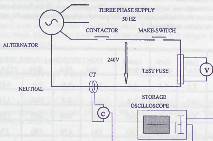
Figure 4. Short circuit arrangement.
