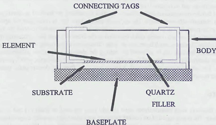
Figure 2 Physical arrangement of the fuselink.
