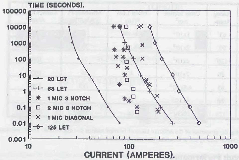
Figure 3 Time Current characteristics
