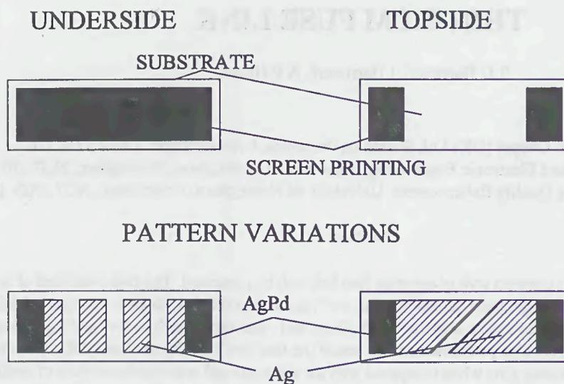
Figure 1 Element Configuration
