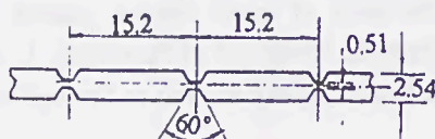
Figure2. The dimension of the Fuse-element
