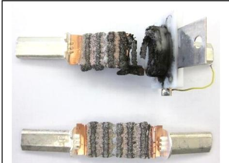
**Fig. 5: Comparison of the tripped fuse elements of a triggered fuse link (up) and a fuse element of an unmodified fuse link (down)**
