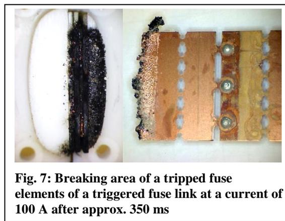
**Fig. 7: Breaking area of a tripped fuse elements of a triggered fuse link at a current of 100 A after approx. 350 ms**
