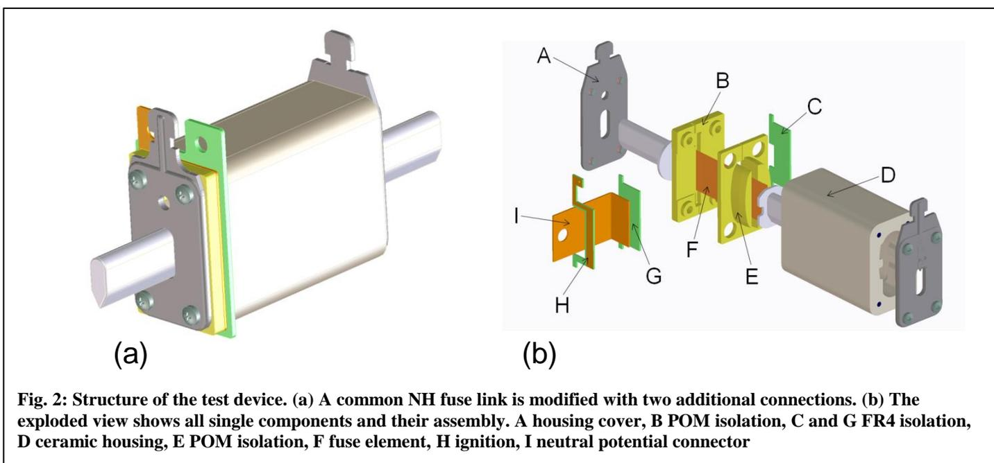
**Fig. 2: Structure of the test device. (a) A common NH fuse link is modified with two additional connections. (b) The exploded view shows all single components and their assembly. A housing cover, B POM isolation, C and G FR4 isolation, D ceramic housing, E POM isolation, F fuse element, H ignition, I neutral potential connector**
