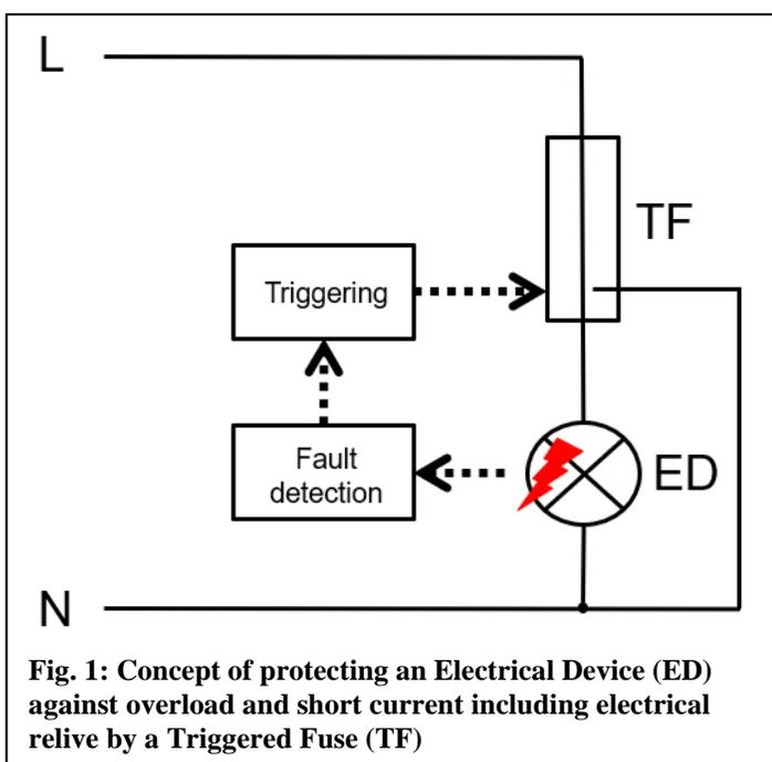
**Fig. 1: Concept of protecting an Electrical Device (ED) against overload and short current including electrical relive by a Triggered Fuse (TF)**
