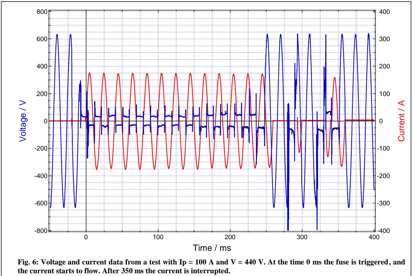
**Fig. 6: Voltage and current data from a test with  $I_p = 100$  A and  $V = 440$  V. At the time 0 ms the fuse is triggered, and the current starts to flow. After 350 ms the current is interrupted.**
