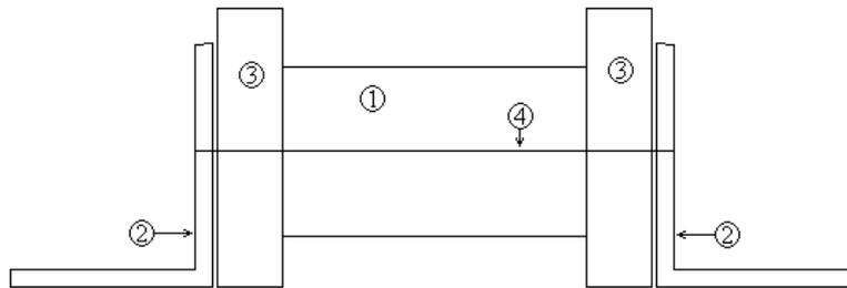
Figure 2. Simplified illustrations of the side view of the test device. Parts: 1) Cavity capable of filling with silica sand, 2) Electrode clamps, 3) Shutters of the filling cavity, 4) Fuse element in copper
