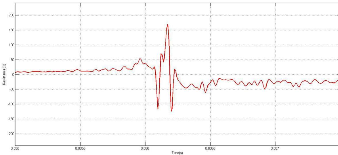
Figure 6. The waveform of the of the fusion process resistance  $R=f(t)$  of the measurement of Fig 5.
