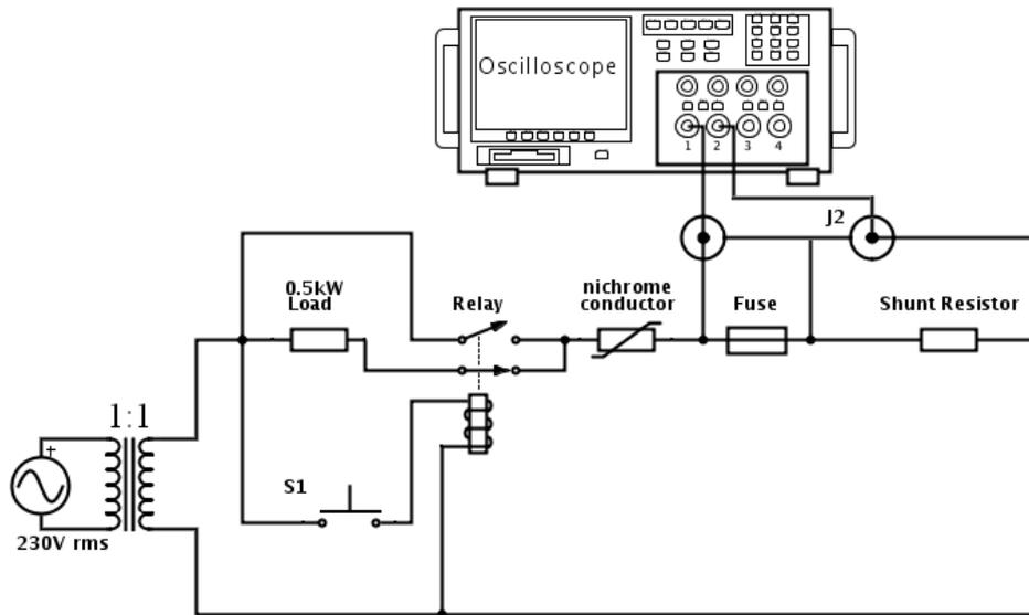
Figure 1. Simplified schematic diagram of the experimental set-up.
