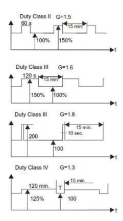
Fig 3 Duty Cycles for defined industrial applications
