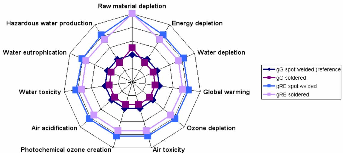
It is clear that for gG-fuses, the soldered solution gives better results for all the points, except for raw material depletion, mainly explained by a higher quantity of copper for the studied solution.
