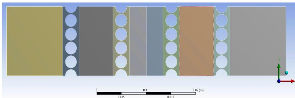
Figure 1. 3D test geometry, subjected to a DC high over-current load (5x rated current).
