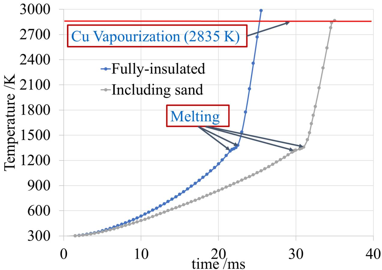
Figure 2. Comparison of numerical results for the temperature variation between fully-insulated vs. sand inclusion cases.
