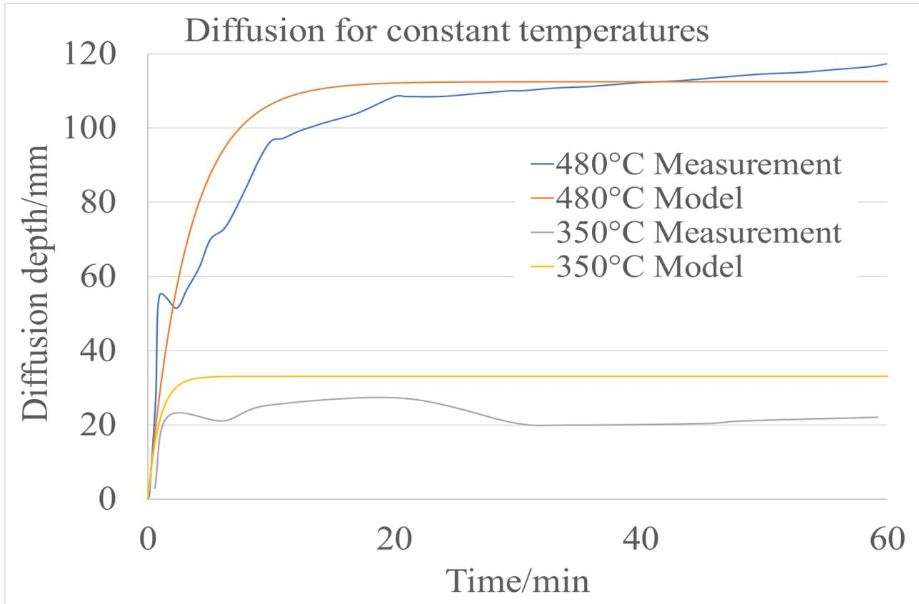
Figure 3. Numerical and experimental results for the diffusion under constant temperature.
