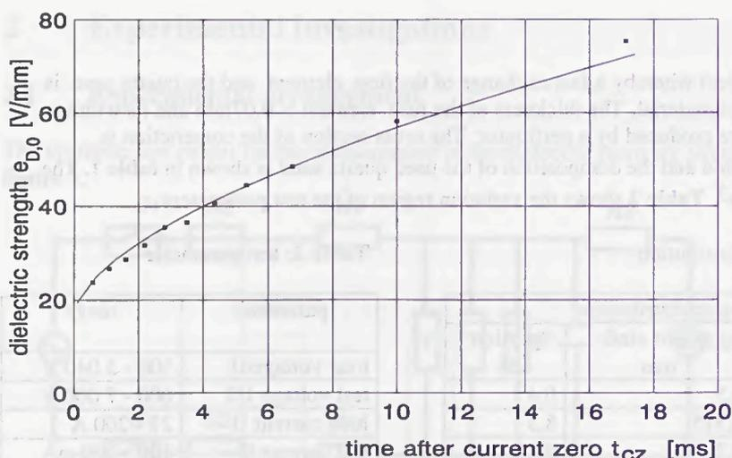
Figure 4: Dielectric strength of the reference experiment versus the time after current zero
