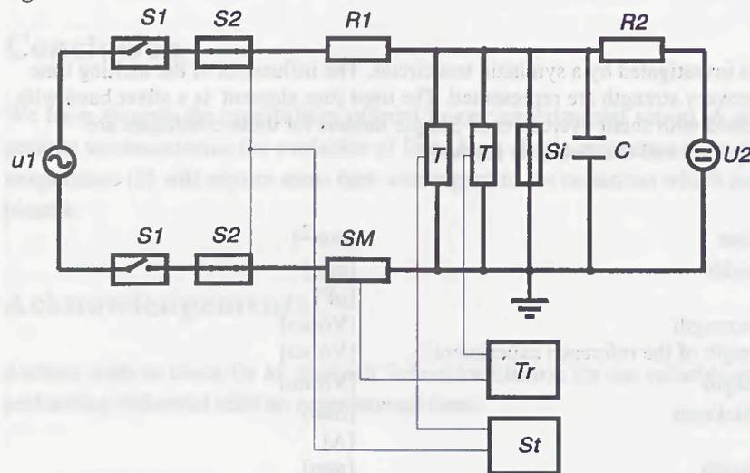
Figure 1: Synthetic test circuit
