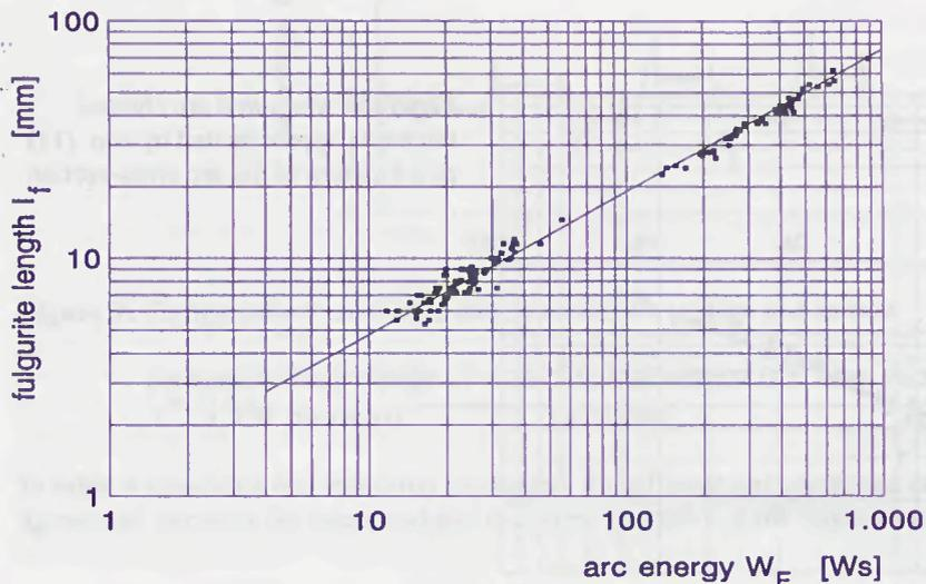
**Figure 7:** Measured fulgurite length approximated by equ. (7) as a function of the arc energy
