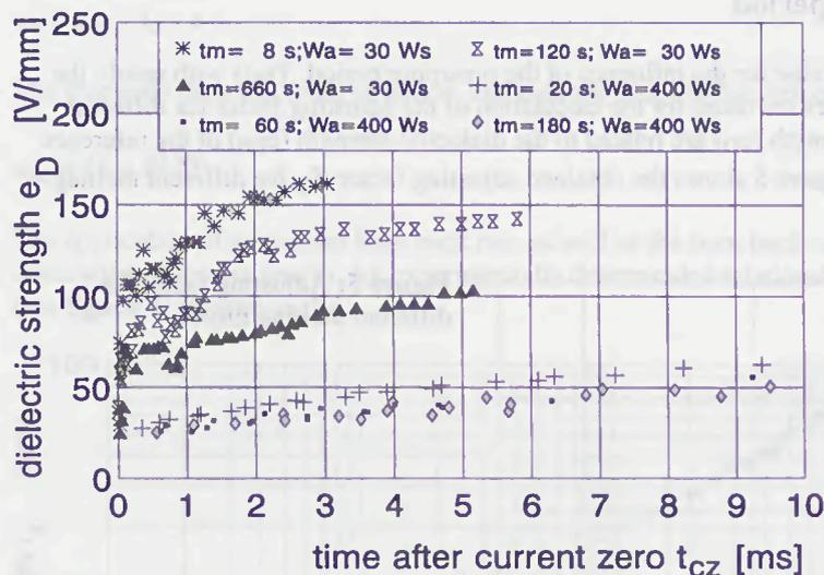
**Figure 3:** Dielectric strength versus the time after current zero
