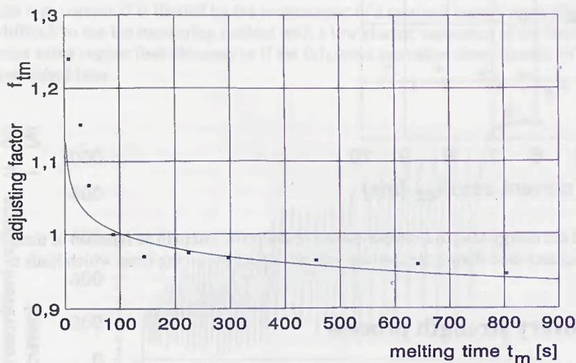
Figure 5: Adjusting factor for different melting times
