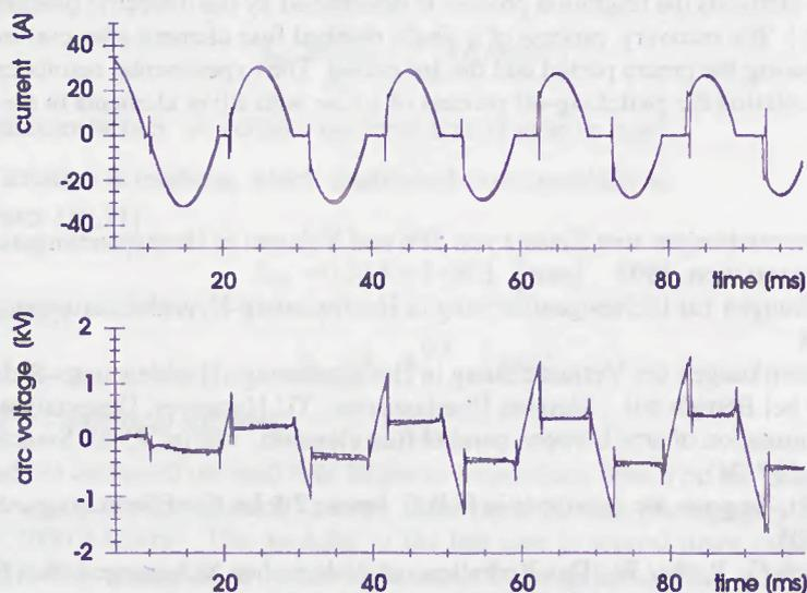
Figure 9: Comparison of calculated and measured arc voltage and current
