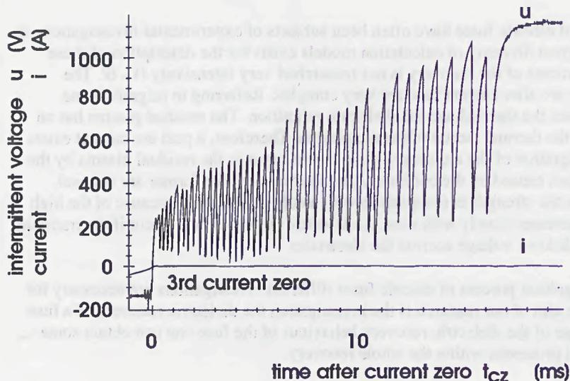
Figure 2: Dielectric breakdown voltage after current zero
