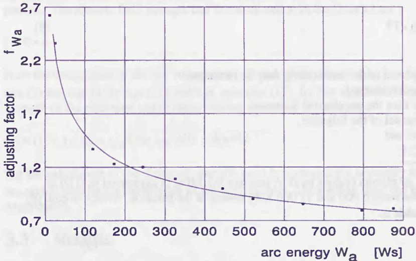
**Figure 6:** Adjusting factor for different arc energies
