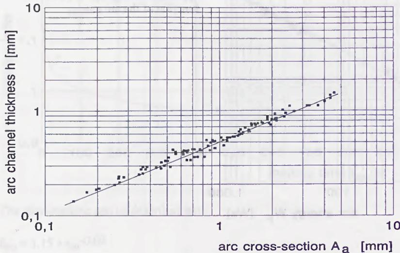
Figure 8: Measured arc channel thickness approximated by equ. (11) as a function of the arc cross-section
