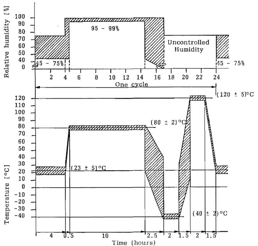
Fig. 4 : temperature and humidity cycle test. The test continues for 10 cycles.
