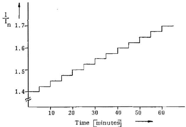
Fig. 3 : "step-test" or "current-test"  $I_n$  is rated current.
