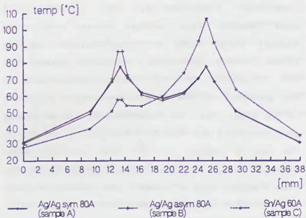
Figure 5 Section View of Fuse Steady-State Temperature Profile of Sample Parallel Elements Types A, B and C
