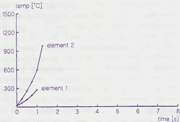
Figure 3 Critical time-current Temperature Rise of Sample C Sn-Ag Strip Elements ( $I = 300A$ )
