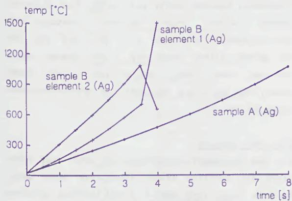
Figure 2 Critical Time-current Temperature Rise of Sample A and Sample B Silver Strip Elements ( $I = 300A$ )
