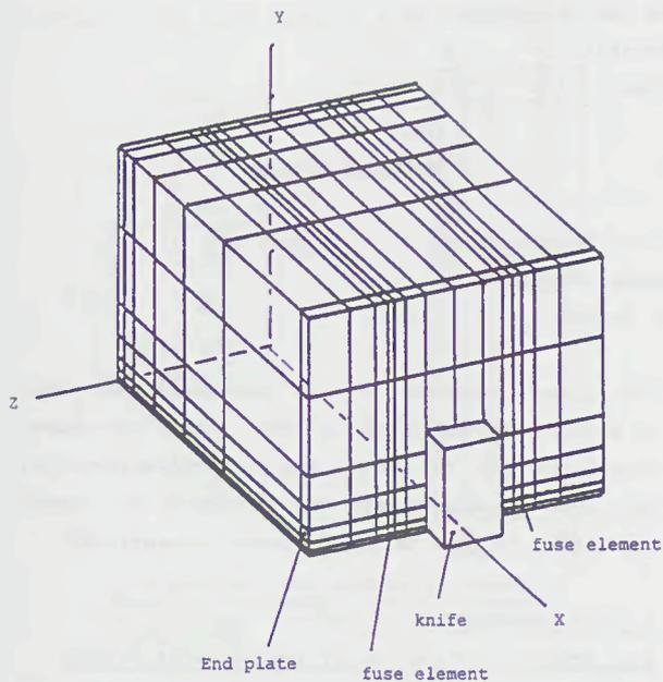
Figure 1 Finite Element Fuse Model
