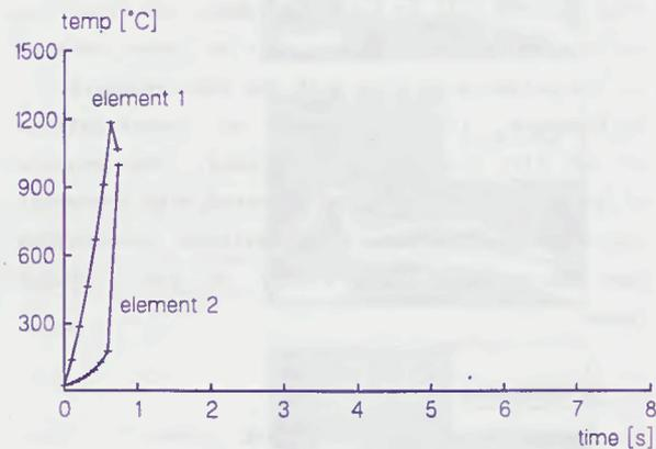
Figure 4 Critical Time-current Temperature Rise of Sample D Ag-Sn Strip Elements ( $I = 300A$ )
