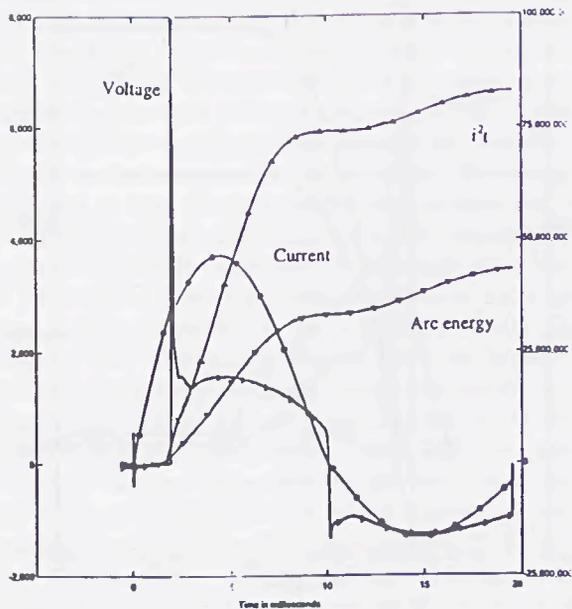
Figure 5: Plots for current and voltage (on left side) and arc energy and arc  $i^2t$  (on right side) for  $B_2O_3$ .
