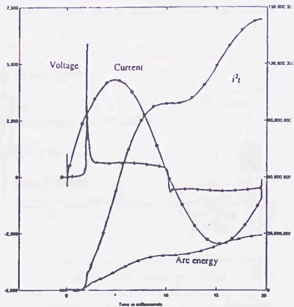
Figure 6: Plots for current and voltage (on left side) and arc energy and arc  $i^2t$  (on right side) for  $ZnO$ .
