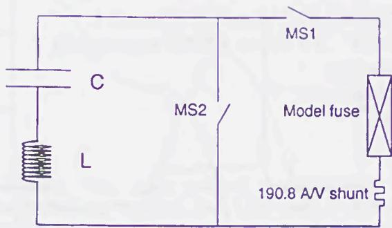
Figure 1: Electrical circuit to energise the test fuse.
