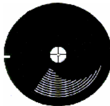
Fig. 6i Patterned-encoded wheel, typical of sequential arc ignition
