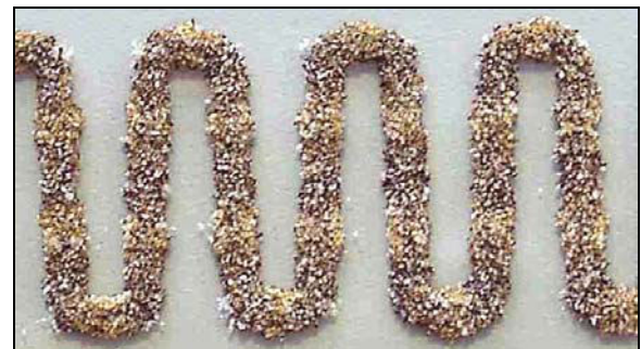
Fig. 12: Fulgurite formed after successful short-circuit current interruption at 12 kV TRV.
