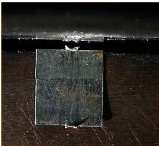
Fig.10 The silver-strip fuse element after 4- \mu s arcing
