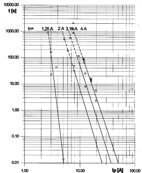
Fig.6: Example of the time-current characteristics of d.c. high-voltage thin-layer fuses.
