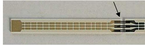
Fig.2: The insulating plate with the deposited fuse-element. The manner of joining of three modules of the fuse-element is indicated by the arrow.
