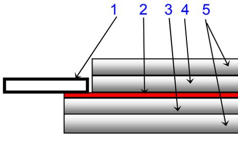
Fig. 1: The sketch of a traction thin-layer fuse after the introduction of the additional insulating cover plates – before air-tight sealing.
