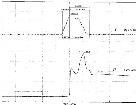
Fig.5: Records of interrupting of the prospective current  $I_1$  of ab. 40 kA, 3.9 kV d.c., time constant 9.9 ms by the traction thin-layer fuse of the rated current of 3.15 A.
