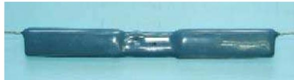
Fig.3: Fuse-element of thin-layer fuse after epoxy resin air-tight sealing.
