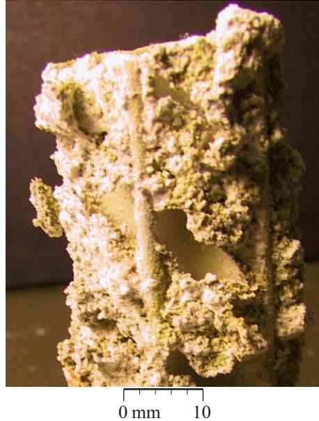
Fig. 13: Fulgurite of a fuse with 30 % of pore filler after  $I_2$ -test.
