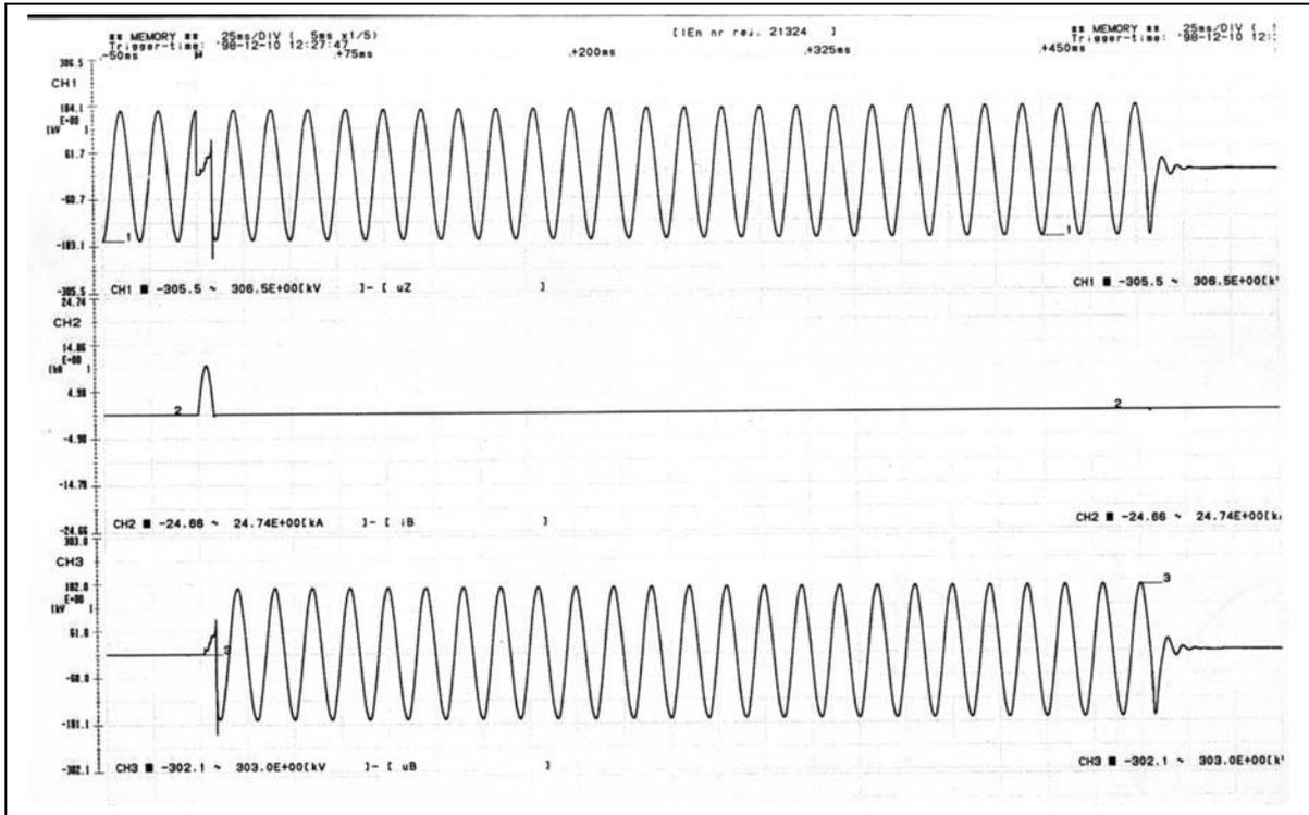
Fig. 7 Breaking capacity test of WZZw-12 High Voltage Protective Assembly, with fuse base PBGw 1-12, fuse carrier OWBGw6-12 and fuse link 40A.
