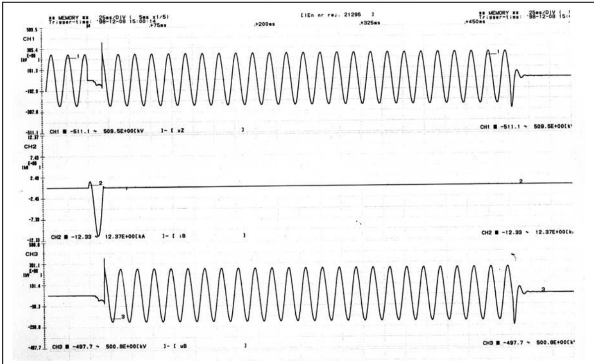
Fig. 8 Breaking capacity test of WZZ-17.5 High Voltage Protective Assembly, with fuse base PBG1-17.5, fuse carrier OWBG2-17.5 and fuse link 40A.
