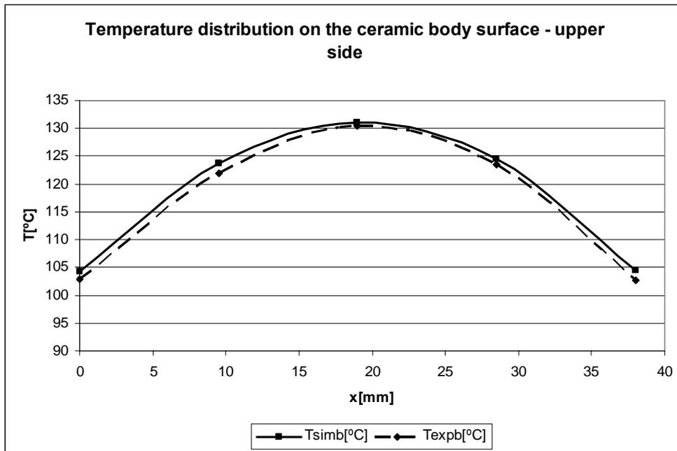
Fig. 9: Comparison between experimental and simulation temperatures vs. length of the ceramic body upper side.
