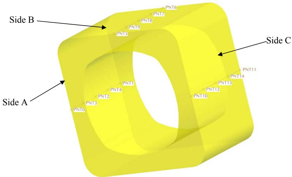
Fig. 7: Measurement points distribution on the surface of the fuse.
