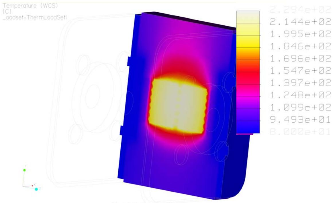
Fig. 5: Temperature distribution through right side fuselink at 75.55% cross section.
