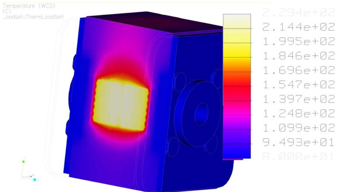
Fig. 3: Temperature distribution through left side fuselink at 24.45% cross section.
