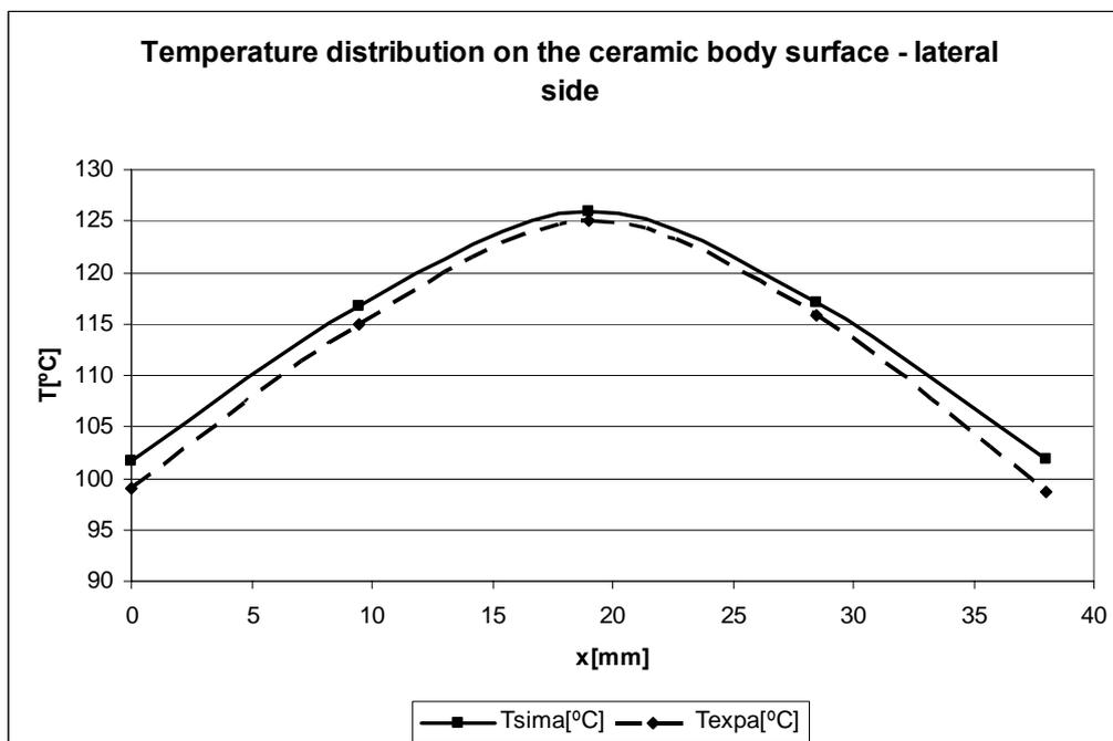
Fig. 8: Comparison between experimental and simulation temperatures vs. length of the ceramic body lateral side.
