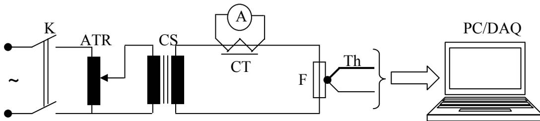
Fig. 6: Experimental tests electrical circuit
