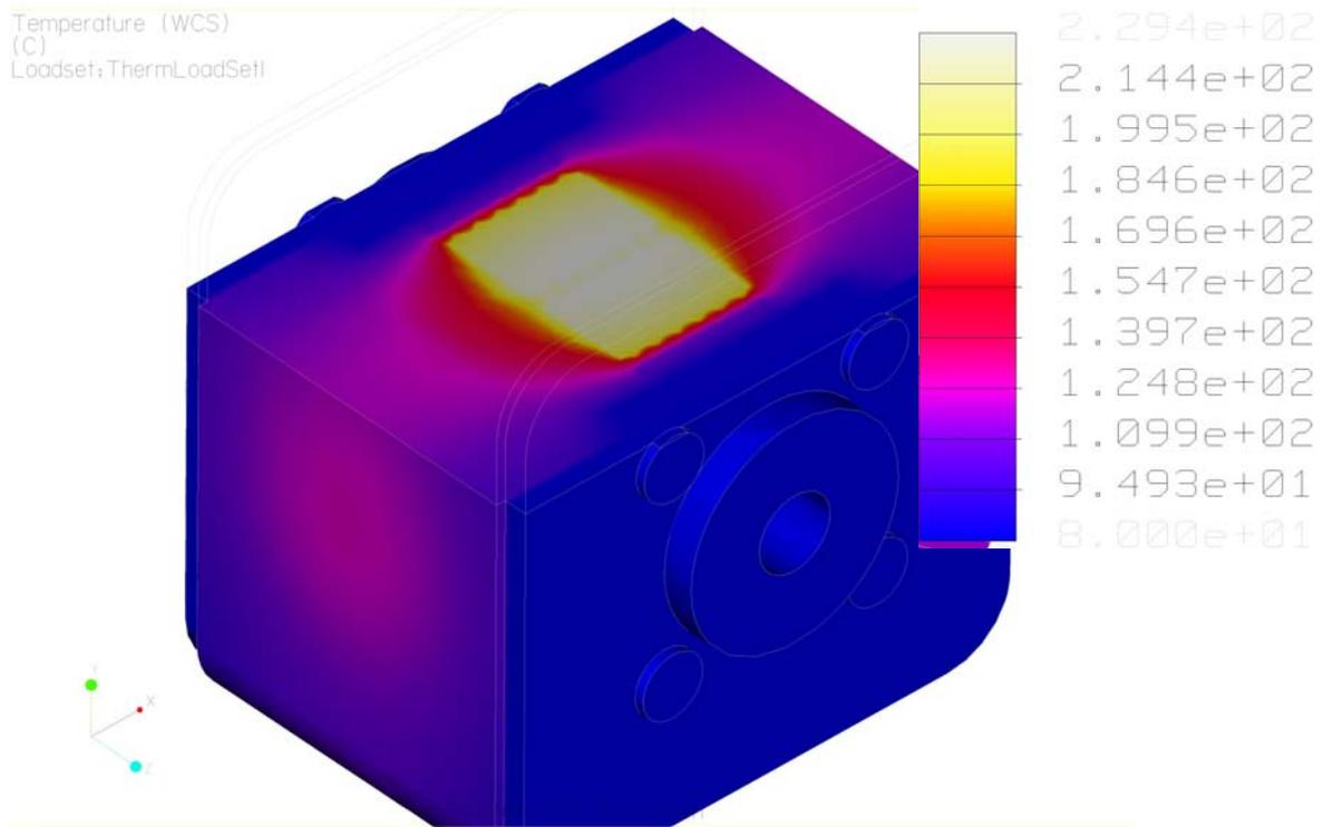
Fig. 4: Temperature distribution through upper side fuselink at 24.45% cross section.
