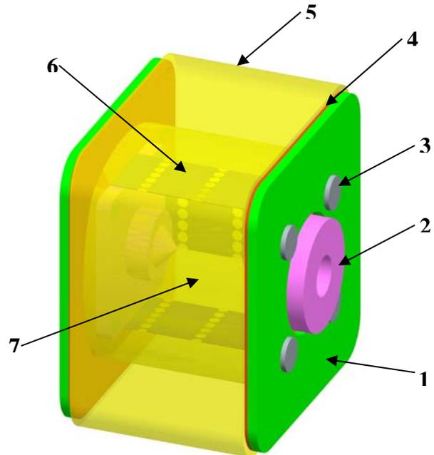
Fig. 1: Thermal model of the fast fuse (1 – outer cap; 2 – end tag; 3 – rivet; 4 – inner cap; 5 - ceramic body; 6 – fuselink; 7 – granular quartz).
