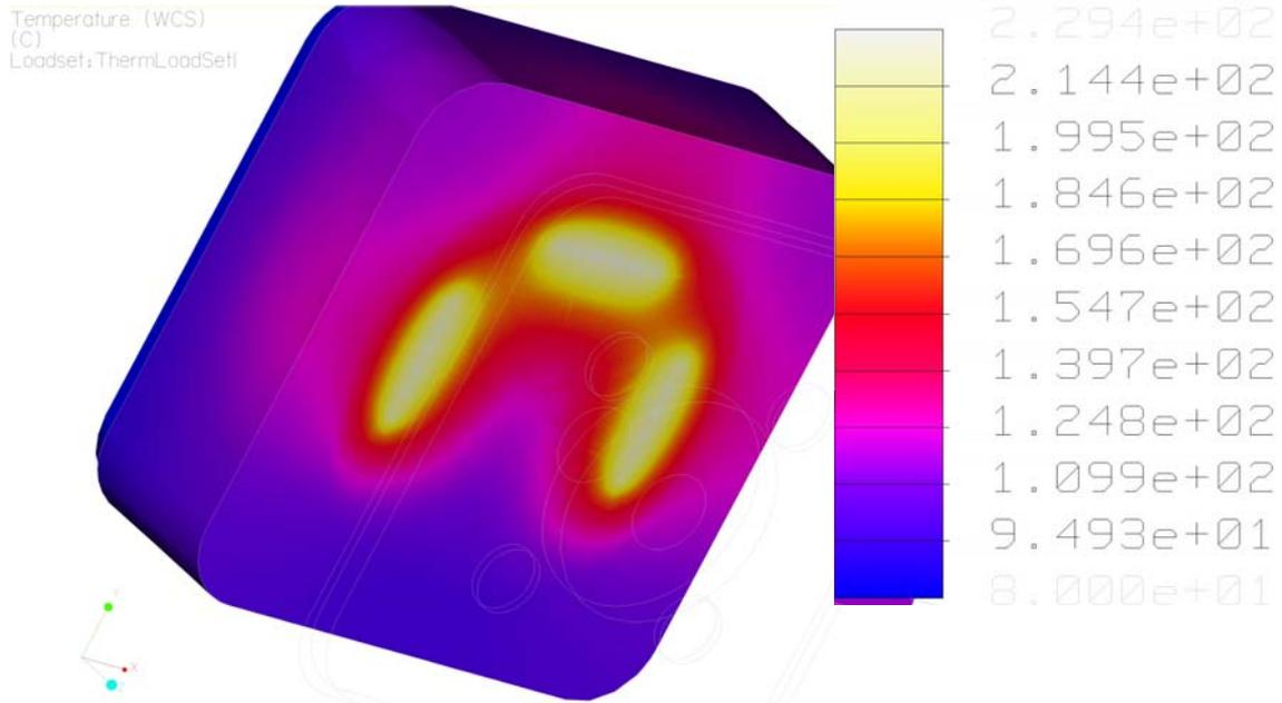
Fig. 2: Temperature distribution through the fuse at 50% cross section.
