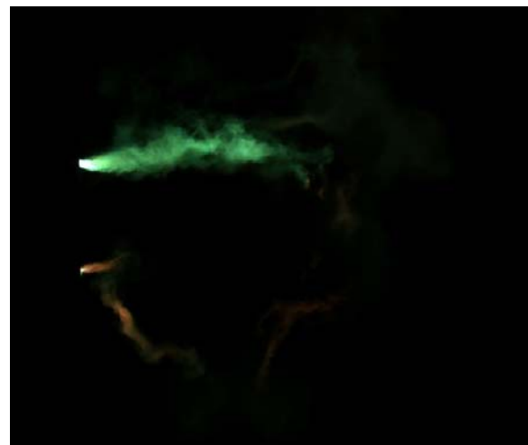
Fig. 2. A frame from a 15kA single phase arc where the lower arc root drifted off the molten copper and produced an air dominated arc jet.
