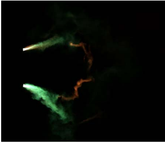
Fig. 3 A single-phase arcing fault showing the electrode vapour oozing out of the constricted column within centimetres of the electrode and an air dominated column connecting the copper dominated arc jets.
