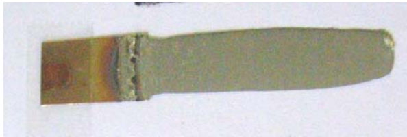
Fig. 3: Test sample strip after dipping illustrates the non uniform dissolution of test strip over its surface.
