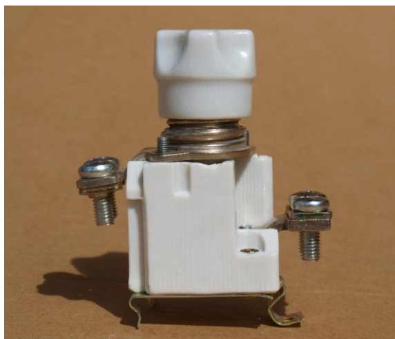
Fig. 2: Size D02 fuse-holder used in tests.
