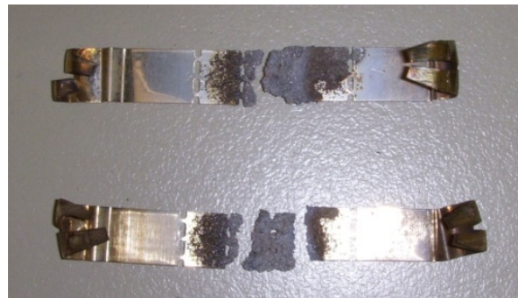
Fig. 9: Melting element after incorrect overload operation
