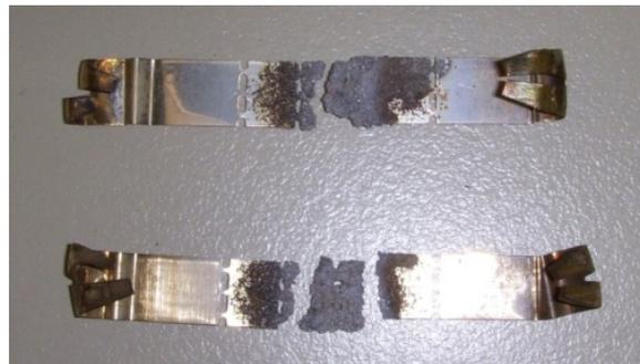
Fig. 9: Melting element after incorrect overload operation
