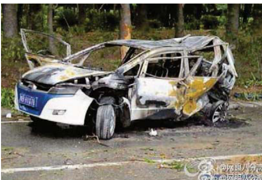
The cause of the massive fire engulfing the e6 was traced to short circuits in the battery pack and wiring, which became highly deformed under strong impact.
