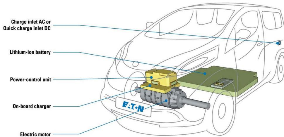
**Fig 4 Typical fuse applications in an Electric Vehicle**
